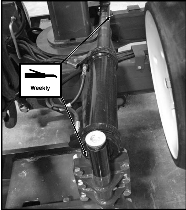
Rotate Cylinder - Grease Weekly 2 fittings
