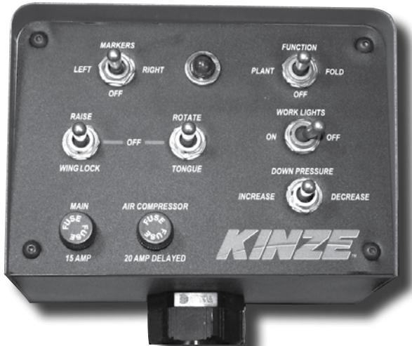
Three Position Selector Switch On Control Console
