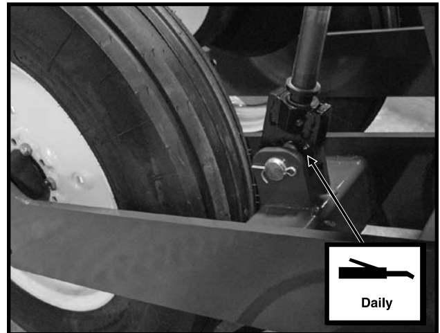
Wing Lift Cylinders - Grease Daily 1 per cylinder 4 cylinders
